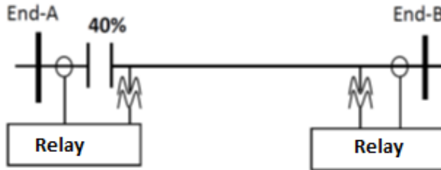
Fig 6: Single circuit with series capacitor located at the end of the line
